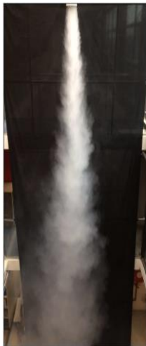
Figure 8: Airflow visualisation of Airius Model 25
