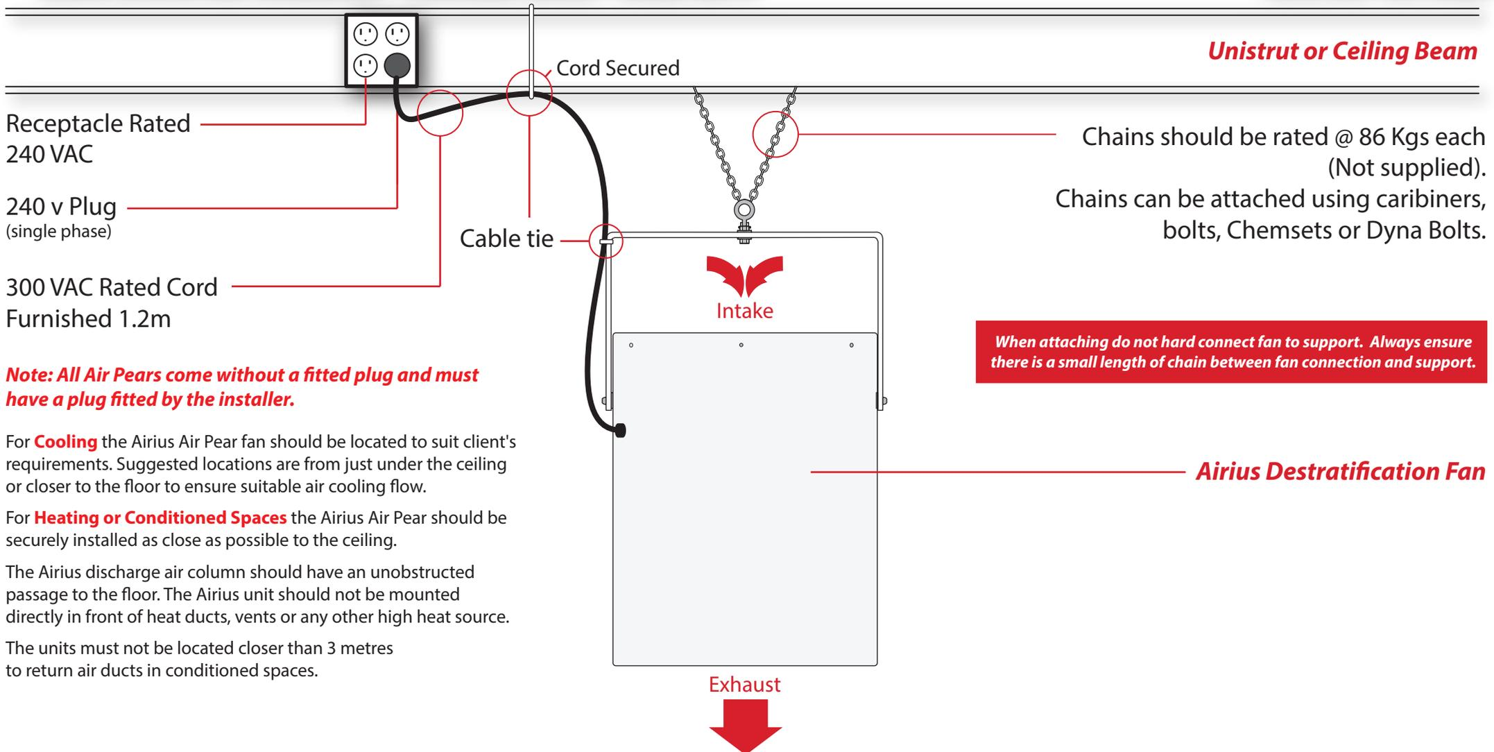
**Note: All Air Pears come without a fitted plug and must have a plug fitted by the installer.**
