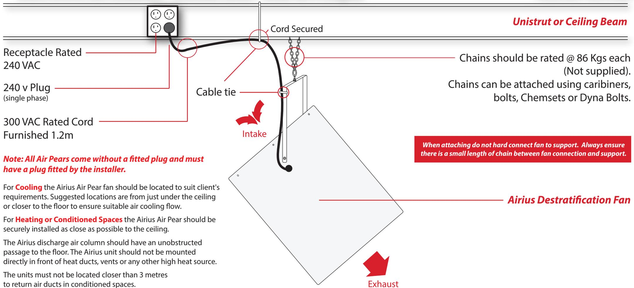
**Note: All Air Pears come without a fitted plug and must have a plug fitted by the installer.**
