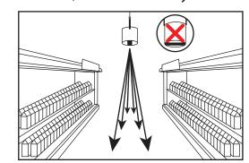
Unit should be positioned with exhaust nozzle parallel to aisle.
