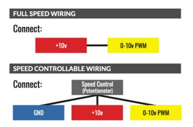
**NOTE:** 0-10 volt analogue signal supplied by fan motor. 3 wire low voltage cable or Cat 5 or Cat 6 cable to be used to either an Airius Potentiometer or a BMS controller (by others).
