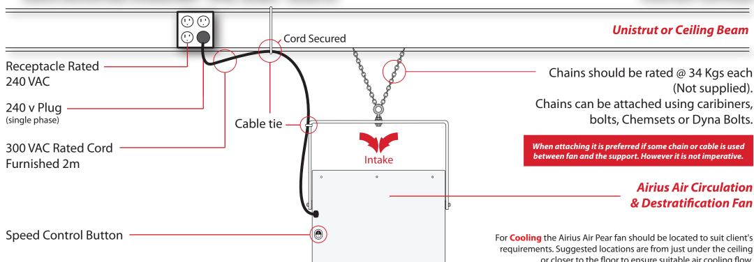
**NOTE:** Includes the option of two speed controls (programmable at factory). Plug can be wired to achieve either high or low speed only, not both, unless plug is required or run a separate control cable in lieu of the switch to a wall mounted switch. Controller by others and easily obtainable at any electrical store. The speeds can be factory programmed if needed.
