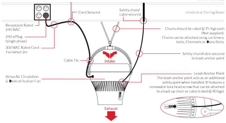
NOTE: Do not hard connect any Airius model 60 fans to structure - use chain (preferred) or cable only
