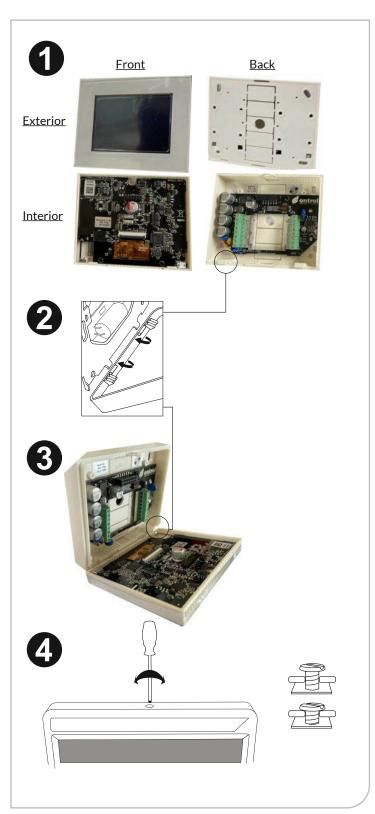
Fit base unit in flush-mounted box.
